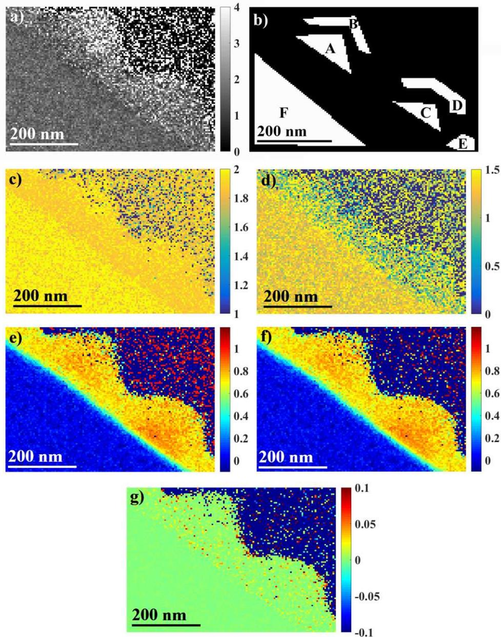
Figure 4: a) Ga K/L ratio map; b) definition of regions masked for histogram analysis; c) map of  $k^*_{\text{InL,GaK}}$ ; d) map of  $k^*_{\text{InL,GaL}}$ ; e)  $x$  map calculated from  $\text{Ga}_K$ ; f)  $x$  map calculated from  $\text{Ga}_L$ ; g)=e)-f) difference map  $\Delta x$  from  $\text{Ga}_K$  and  $\text{Ga}_L$  lines.
