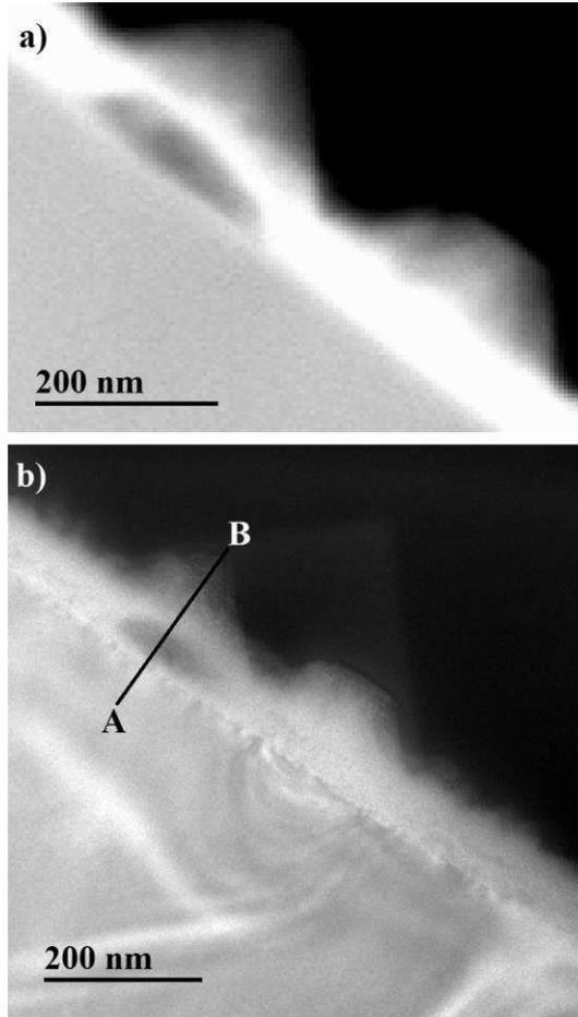
Figure 1: a) ADF image and b) relative thickness map ( $E_0=300\text{kV}$ ,  $\beta=25\text{mrad}$ ,  $\min=0.30$ ,  $\max=3.73$ , where  $t/\lambda=1.0$  in the faintly visible square of carbon contamination) from EFTEM, with position for line profile in Figure 2 as indicated.
