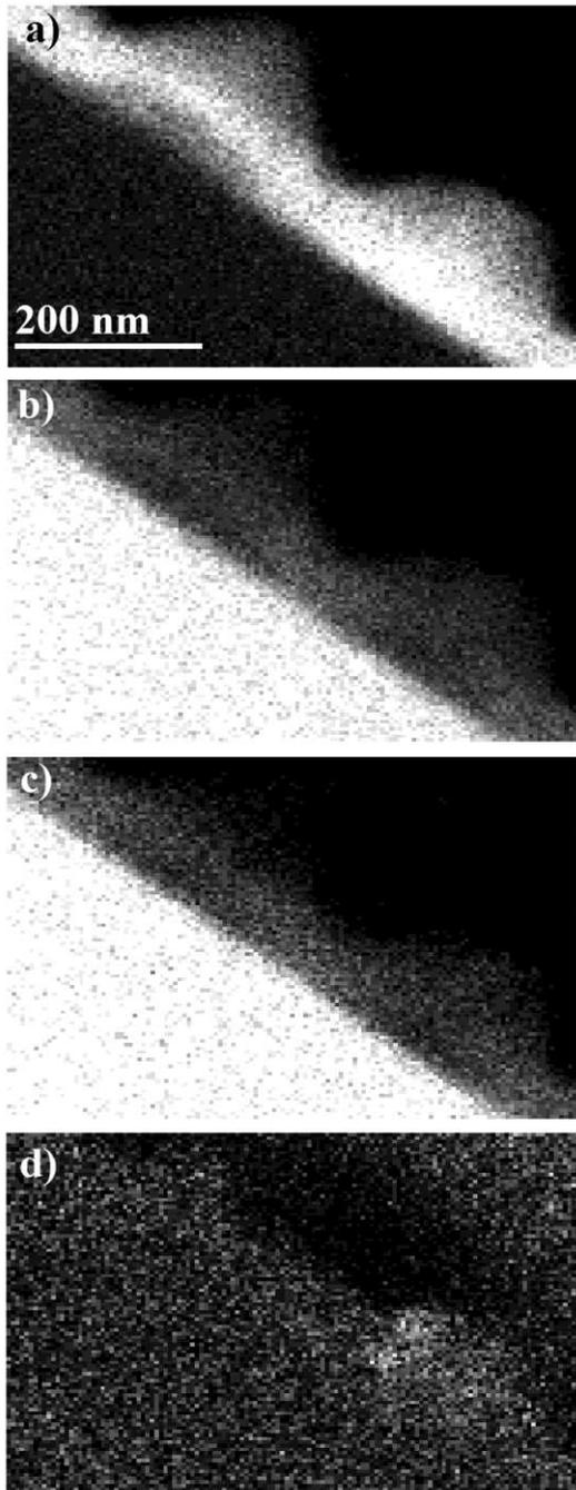
Figure 3: Elemental maps after background subtraction for a)  $\text{In}_L$  ( $\text{In}_L^{\text{max}}=60$  counts); b)  $\text{Ga}_K$  ( $\text{Ga}_K^{\text{max}}=70$  counts); c)  $\text{Ga}_L$  ( $\text{Ga}_L^{\text{max}}=40$  counts); d)  $\text{N}_K$  ( $\text{N}_K^{\text{max}}=11$  counts).
