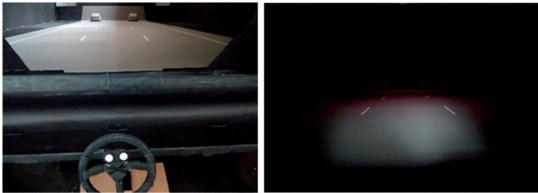
Figure 2. Left: The participant’s view of the road ahead, showing the detection-response buttons on the steering wheel. Right: the view ahead as lit only by the driver’s headlights. Note: laboratory lighting switched on for left-hand photograph to reveal the steering wheel: this lighting was switched off during all trials.
