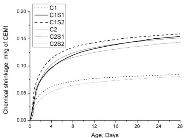
Figure7: Chemical shrinkage normalized to CEM I content
