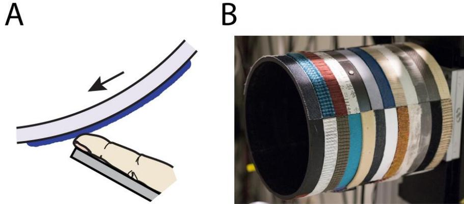
**Figure 2. Experimental setup.** **A.** Textures were passively scanned over the fingertip at 40, 80, 120, and 160 mm/s. **B.** Textures were scanned at a precise speed across the skin with a contact force of 0.3 N using a custom-built drum stimulator.
