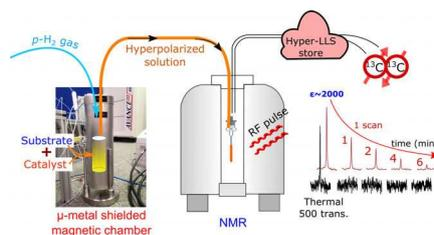
**Only time will tell:** A fast and cost-effective method to increase carbon-13 NMR sensitivity by three orders of magnitude is detailed for a series of pyridazine derivatives. When the resulting polarization is stored as long-lived singlet order, the resulting hyperpolarized  $^{13}\text{C}$  NMR signals remain detectable for up to 10 minutes.
