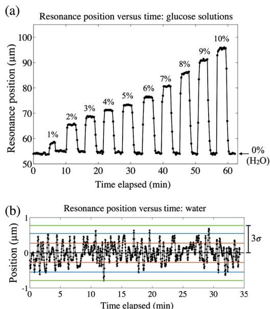
**Fig. 3.** (a) Position of the resonance peak versus time as different glucose solutions are introduced, where the percentages indicate the %w/v glucose concentration. Water (0%) was introduced between each sugar solution. (b) Position versus time for water only, centered about the mean. The red, blue, and green lines indicate one, two, and three standard deviations ( $\sigma$ ) away from the mean, respectively.
