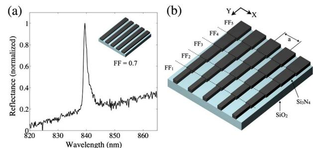
**Fig. 1.** (a) Typical measured reflectance spectrum from a regular  $\text{Si}_3\text{N}_4$  grating. (b) The chirped grating design: the grating is composed of strips, each with a different FF, in order to chirp  $\lambda_R$  as a function of its position along  $Y$  (FF change is exaggerated here for illustration purposes).
