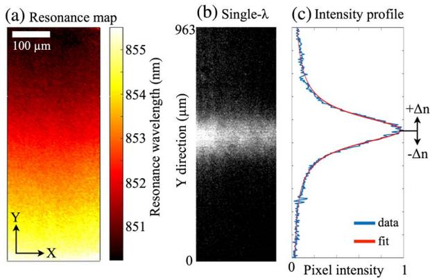
**Fig. 2.** (a) Resonance wavelength map of the grating (water is the surrounding liquid). (b) Brightfield image of the grating under monochromatic illumination. (c) Intensity profile of the resonance shown in (b), averaged horizontally and normalized. The blue curve shows raw data, while the red curve shows a fitted Fano curve, as described in the text. The position of the resonance is monitored continually, allowing changes in the refractive index ( $\Delta n$ ) to be detected.
