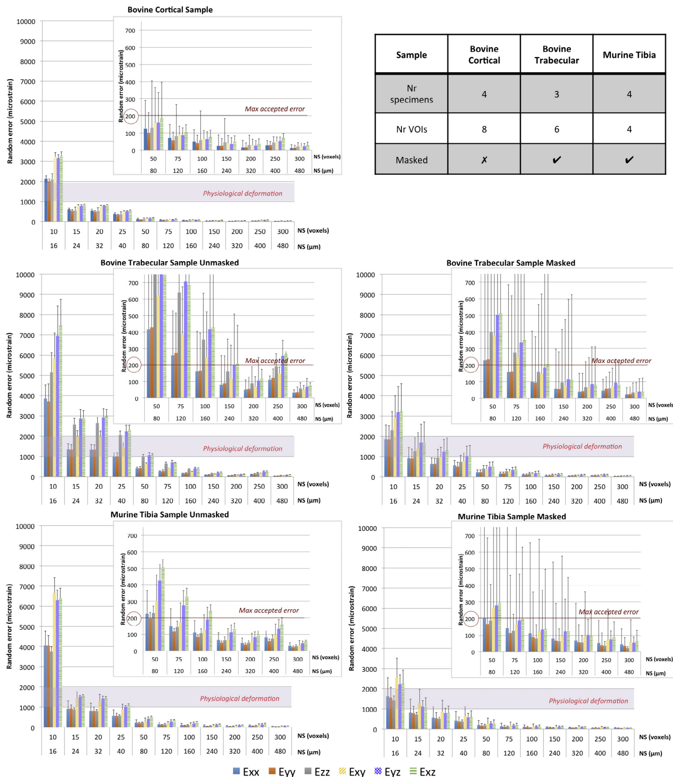
Fig. 5. Median of the random error for each bone type (cortical bone on the top, trabecular bone in the middle and murine tibiae on the bottom), for each registration methods (from unmasked images on the left, from masked images on the right), for each component of strain, as a function of NS. To improve the readability, error bars representing standard deviations were reported only on the top of each histogram. To help interpreting the results, a range for the typical physiological deformations (1,000–2,000 microstrain Yang, et al., 2011) is indicated. For the scope of this study, also the target value for the measurement error is indicated (one order of magnitude lower: 200 microstrain).
