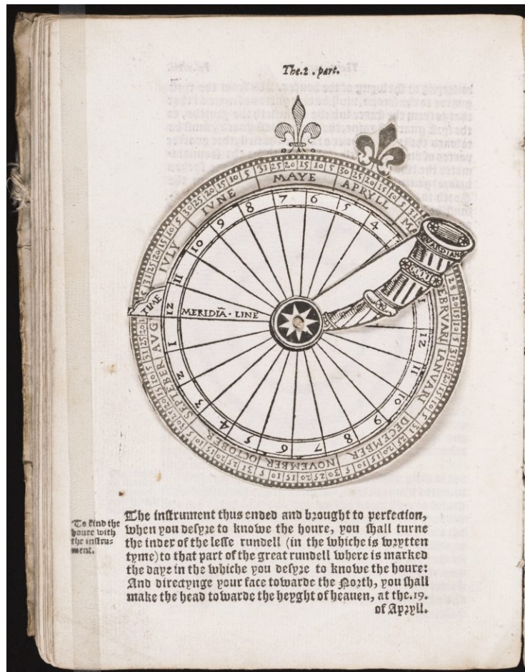
Figure seven: Volvelle, from Martin Cortes, The arte of navigation, conteynng a compendious description of the sphere, with the making of certen instruments and rules for navigations ([London], 1561). Beinecke Library Taylor 129. By permission of the Beinecke Rare Book and Manuscript Library, Yale University.
