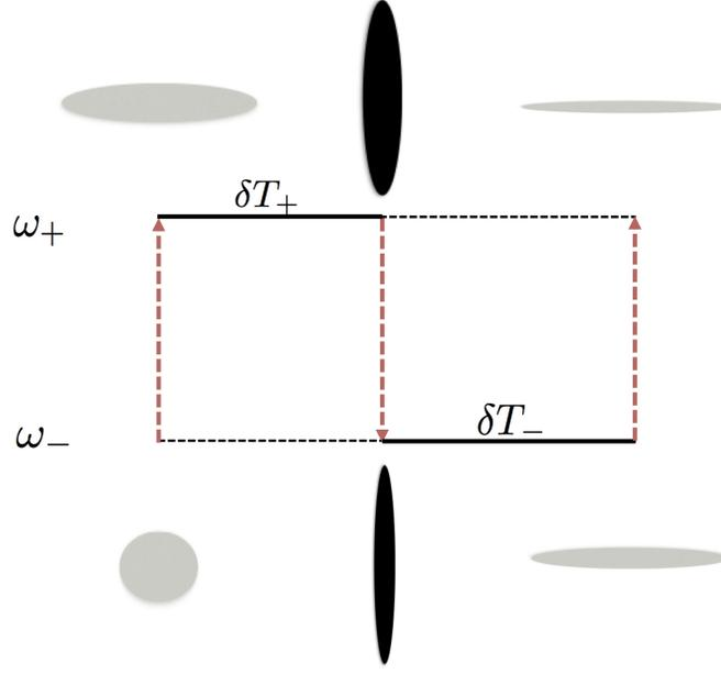
**Figure 3.** (Color online) Schematic of the dispersive squeezing protocol outlined in the text. Heavy dashed arrows represent qubit flips, while solid lines indicate time evolution under the corresponding oscillator Hamiltonian. The ellipses illustrate the state of the field before and after each qubit flip. One full cycle plus the first step of a second is shown here.
