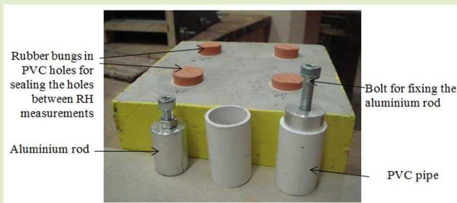
**Fig. 1.** Concrete blocks of size 150x150x80mm along with PVC inserts and various attachments used to create holes for monitoring the internal RH values
