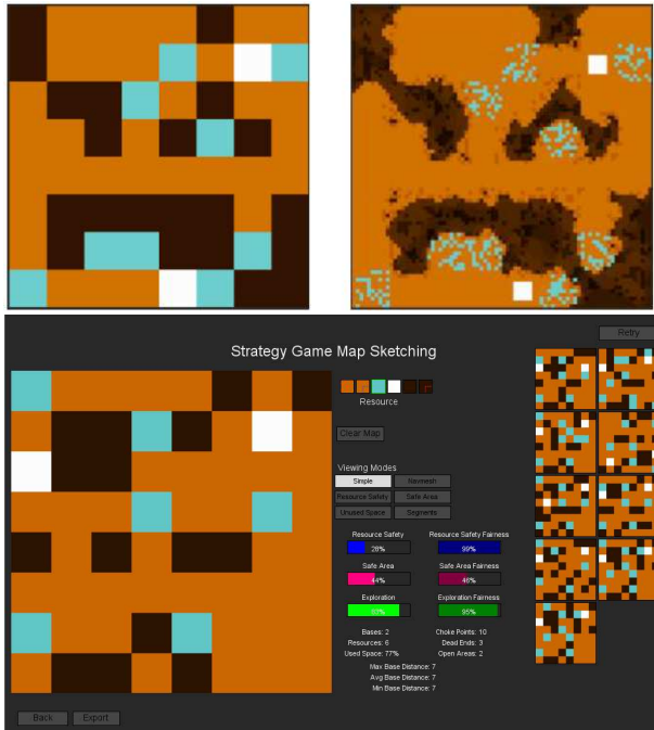
Figure 4: Sentient Sketchbook, a MICI game map generator: the designer creates a low-detail map, the AI evaluates its playability and evolutionarily generates better alternative suggestions, which the designer can then choose and modify. The AI can turn any low-detail into a high-detail map [23].
