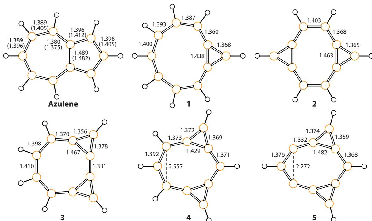
Figure 2: MP2(Full)/cc-pVTZ optimized ground state geometries of azulene and compounds 1–5 (azulene and 1, 3–5:  $C_{2v}$  symmetry; 2:  $D_{2h}$  symmetry). Symmetry-unique bond lengths and other distances in Å; the experimental bond lengths in azulene [13] are given in brackets, rounded to three decimal places.
