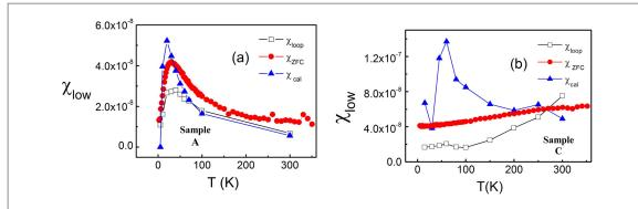
**Figure 3.** Low-field susceptibilities (a) for sample A and (b) for sample C. Black open squares, as measured directly from the hysteresis loop; red circles, from the ZFC plot; blue triangles, as calculated from the measured values of the remanence using equation (2).
