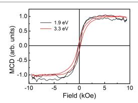
**Figure 6.** MCD hysteresis loops measured at room temperature for sample C at energies 1.9 and 3.3 eV. The paramagnetic contribution due to the MCD from the substrate has been subtracted from the plots and the plots scaled to the same value at saturation.
