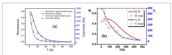
**Figure 4.** The temperature variation of the coercive field,  $H_C$ , (triangles) and the reduced remanence,  $M_r/M_s$ , (squares) for samples A in (a) and C in (b). The symbols are data derived from SQUID magnetometry. The curves are obtained from the theoretical model of independent Co particles this is presented in appendix with parameters chosen to fit  $H_C$ .
