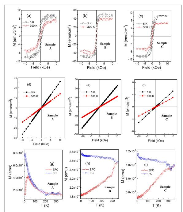
**Figure 2.** (a) (b) and (c) show the hysteresis loops at 300 K and at low temperature for samples A, B and C respectively where the contributions of both the diamagnetic substrate and the residual paramagnetism, have been subtracted. The residual paramagnetic susceptibility is shown in figures (d), (e), (f). The zero-field-cooled and field-cooled magnetizations are shown in figures (g), (h) and (i). Samples A and B were measured in 100 Oe and sample C in 200 Oe.
