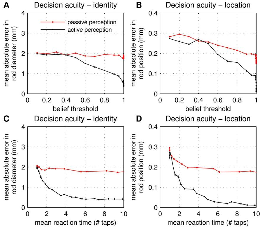
**Fig. 7.** Decision acuity for active and passive perception. (A,B) Dependence of the mean absolute errors of rod diameter and position plotted against the ‘what’ belief threshold. Passive perception is shown in red and active perception in black. (C,D) Dependence of these perceptual acuities instead plotted against mean reaction time (with belief threshold an implicit parameter determining all quantities).
