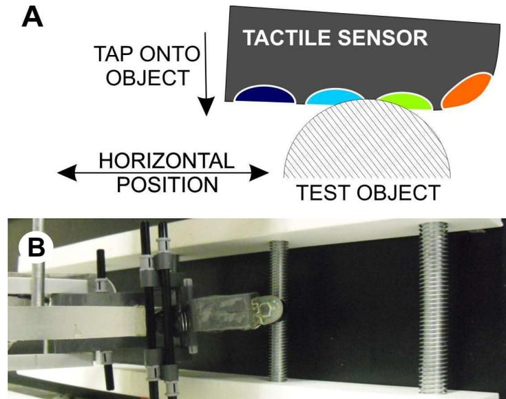
**Fig. 1.** Experimental setup. (A) Schematic of tactile sensor contacting a cylindrical test object. The fingertip is moved horizontally to sample object contacts from different positions. (B) Top-down view of experiment, with the fingertip mounting on the arm of the Cartesian robot visible to the left.
