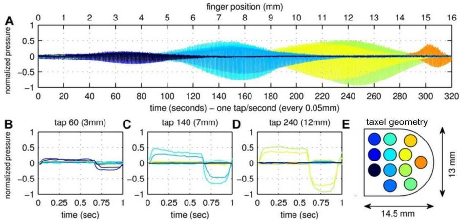
**Fig. 3.** Fingertip pressure data recorded as the finger taps against a test rod (diameter 4 mm) at a constant rate of 1 tap/sec. The range of finger positions spanned 16 mm over 320 s, giving 320 taps spaced every 0.05 mm. Tickmarks are shown every 1 mm displacement, or 20 taps. Data from the different taxels are represented in distinct colors depending on the taxel position shown on the diagram to the right.
