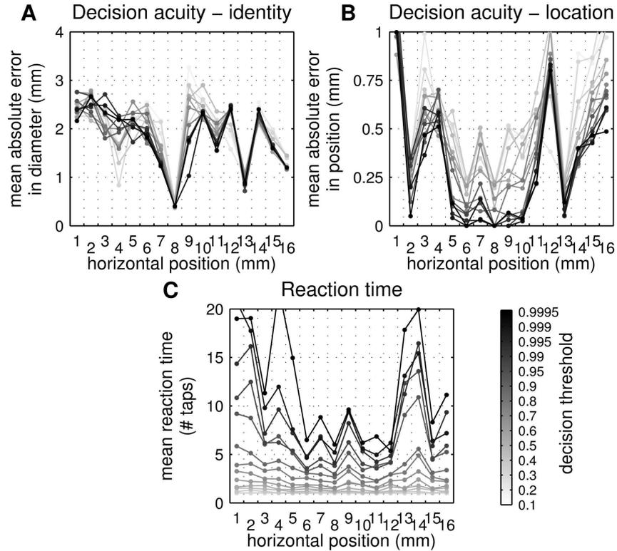
**Fig. 5.** Active perception results depends on the decision threshold and fixation point. The mean accuracy of identifying the cylinder (A) and the mean reaction time (B) vary with threshold (gray-shade of plot) and fixation point ( $x$ -axis). Each data point corresponds to 1000 decision trials.
