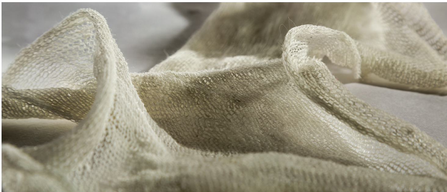
1 Programmable Knitting: the knitted surface actuates causing waves of movement along the fabric length. (Scott, 2015 © )
