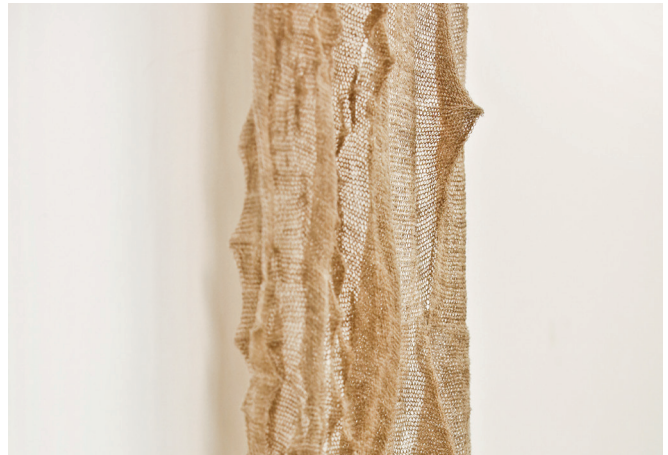
11 Fabric actuated using cold water spray (Schek, 2015 ©)
