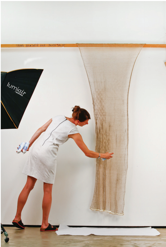
11 Fabric actuated using cold water spray (Schek, 2015 ©)
