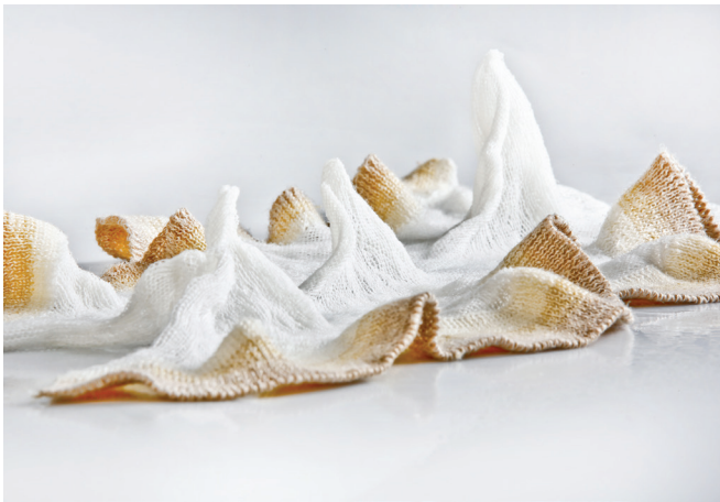
3 Programmable Knitting: after actuation fabric forms spiral peaks (Schek, 2015 ©)
