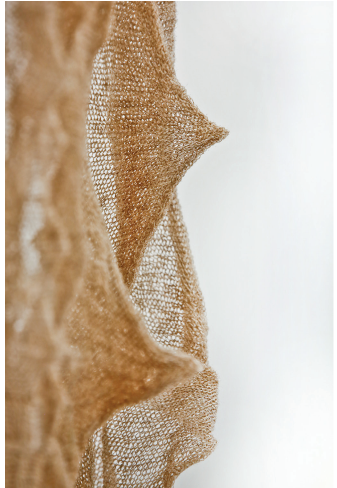
4 Skew: Detail of knitted surface after actuation in 3D/wet state. (Schek, 2015 ©)
