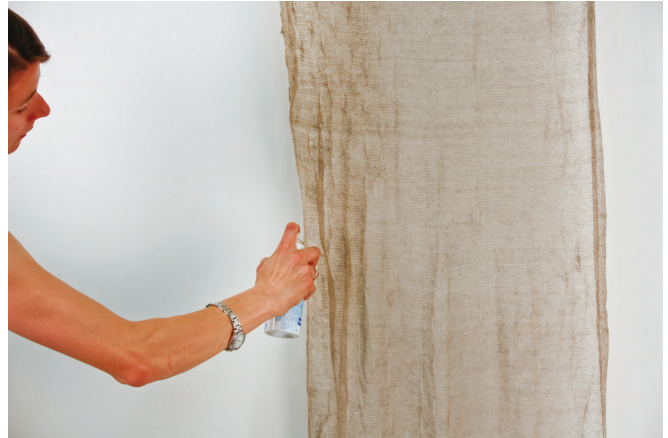
11 Fabric actuated using cold water spray (Schek, 2015 ©)
