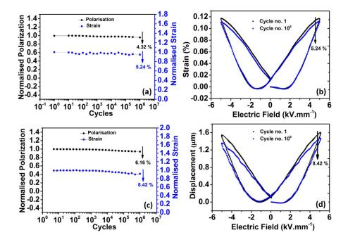
FIG. 4. (a) Polarization and strain for bulk KBNFT9 ceramics as a function of switching cycle; (b) S-E loops for KBNFT9 bulk ceramics at 1st and millionth cycle at 10 Hz; (c) polarization and strain for a KBNFT9 MLA as a function of switching cycle; and (d) comparison of S-E loops for KBNFT9 MLA at 1st and millionth cycle at 5 Hz.
