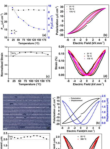
FIG. 2. (a) Maximum and remanent polarization versus temperature for KBNFT9 bulk ceramics; (b) P-E loops for KBNFT9 bulk ceramics at different temperatures: (c) normalised bipolar strain versus temperature for KBNFT9 bulk ceramics; and (d) S-E loops for KBNFT9 bulk ceramics at different temperatures.
