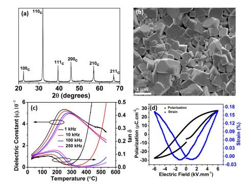
FIG. 1. (a) XRD pattern of KBNFT9 at RT; (b) the ceramic microstructure of KBNFT9; (c) permittivity and  $\tan \delta$  versus temperature for KBNFT9 ceramics; (d) P-E and S-E loops for KBNFT9 bulk ceramics at RT and at a frequency of 1 Hz.
