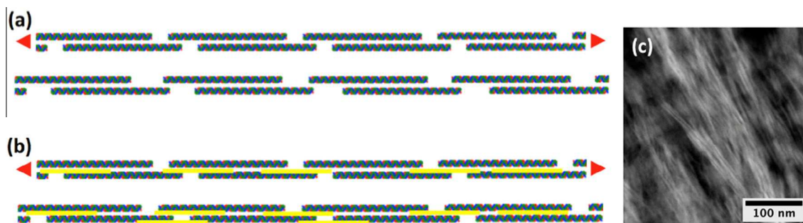
Fig. 8. Schematic illustrating the role of increased degree of mineralization in the enhanced stiffness of collagen. (a) Unloaded and loaded case of non-mineralized collagen showing the gap region between the triple collagen helices expanding. (b) Unloaded and loaded case for mineralized collagen (mineral phase in yellow) showing the mineral nanocrystals interlocking the triple helices. (c) Apatite crystals in the collagen matrix of human bone as observed by STEM. (For interpretation of the references to colour in this figure legend, the reader is referred to the web version of this article.)
