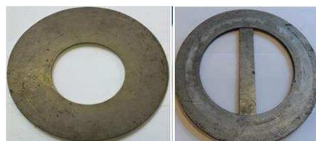
**Figure 1.** Turbulent generating obstacles – hole type (left), flat bar type (right).
