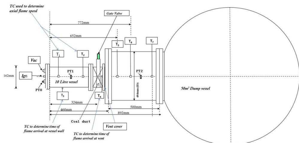
Figure 2: Experimental set-up for vented explosions.
