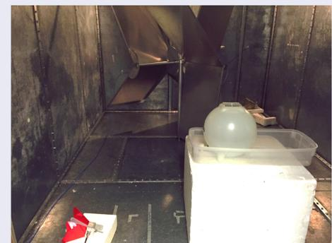
Figure: the ACS measurement in reverberation chamber
