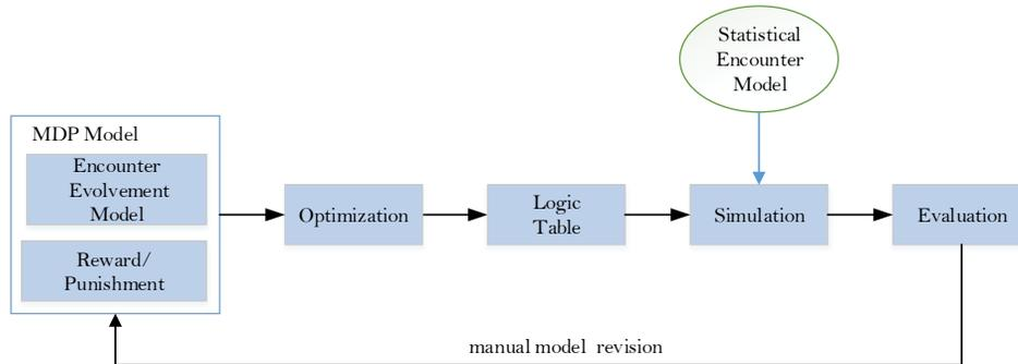
Fig. 1. ACAS  $X_U$  development process, adapted from [1].
