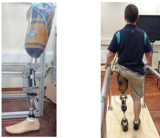
(a) LPK attached to a commercial prosthetic foot and custom-made socket (b) LPK system attached to TFA Fig. 7. LPK connected to a TFA.
